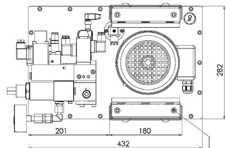
M8 thread for lifting devices
