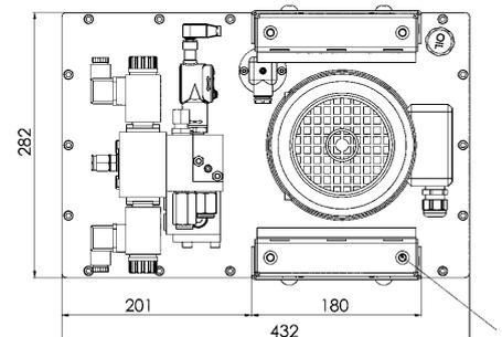
M8 thread for lifting devices
