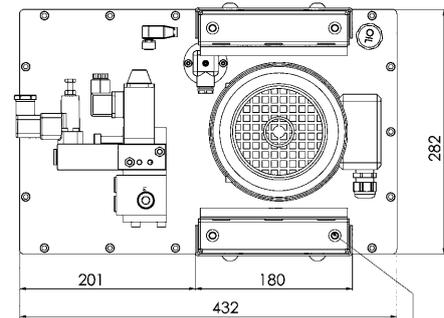
M8 thread for lifting devices
